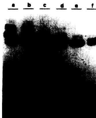
Figure 6. PAGE (20%, 8 M urea) profile of oligonucleotides 11-13 . Lanes b, d, f correspond to 11-13 respectively prepared using PNT methyl phosphonamidites. The lanes a, c, e correspond to 11-13 respectively, prepared using commercial methyl-phosphonamidites.
